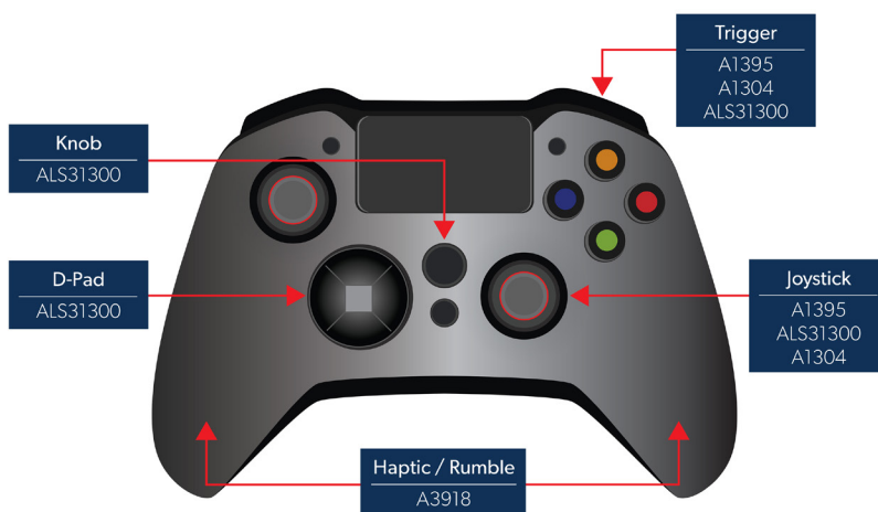
Figure 1: Common controller functions enabled by magnetic sensors.
